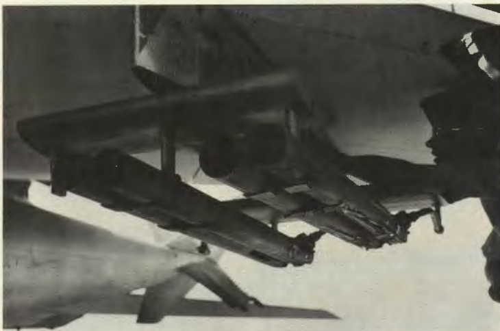
Close-up shows minor damage to rocket tubes.
